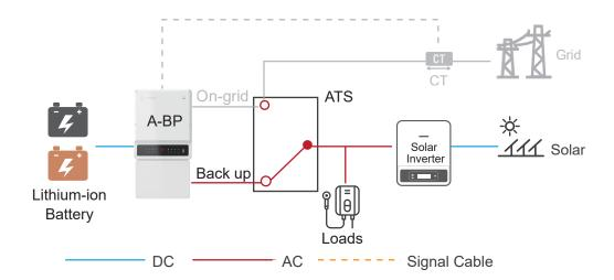
When grid is available, grid-tied inverter AC output connect to the on-grid port of ABP through ATS. Solar power of the system will support loads first then charge battery, and the exceed power will be able to export to grid which could be limited. If the solar power is not enough to support loads, battery will discharge.
