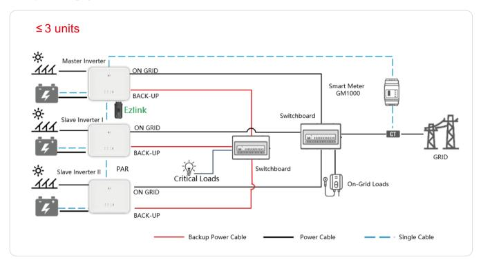
3-unit paralleled system can reach a maximum total power of 18kW. What's more,it can realize a UPSlevel switching from on grid to off grid mode within 10ms.
